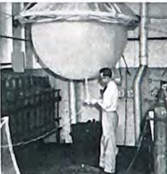
Fitting radar target to the met. balloon. Once in the upper air the balloon bursts, the radio-sonde equipment descends by parachute
