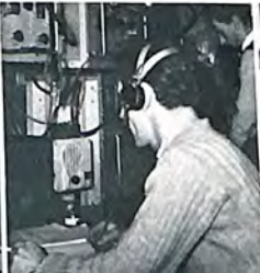
Readings are signalled back to the ship by the transmitter in the met. balloons, and are later signalled to land stations
