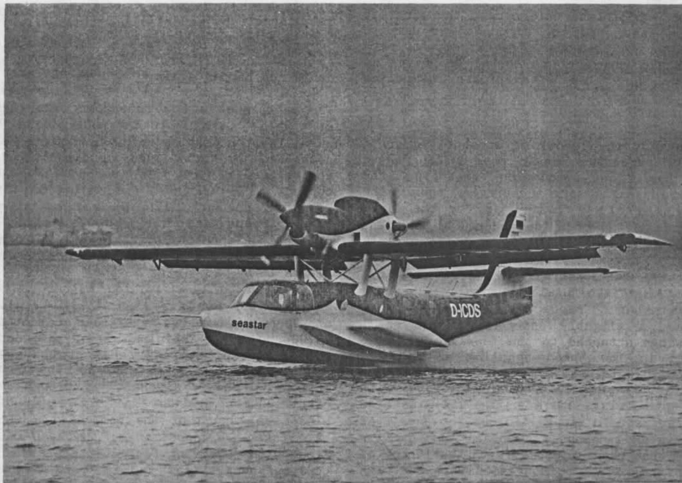
THE CLAUDIS DORNIER SEASTAR DURING WATER TRIALS, CLEARLY SHOWING THE TWO STEP FLAT BOTTOMED HULL, SIDE SPONSON AND STUB WING (C. D. S. GmbH via STUART BOURNE)
